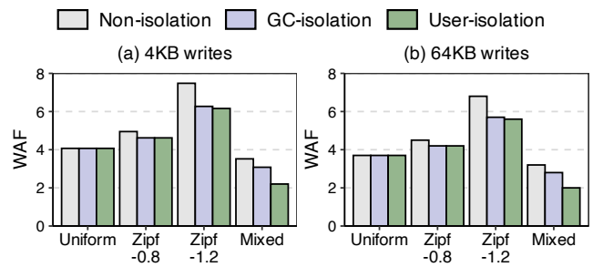
Figure 18. CSAL GC Write Amplification. User-isolation means adding user-isolation with GC-isolation, which enables both GC-isolation and user-isolation.
