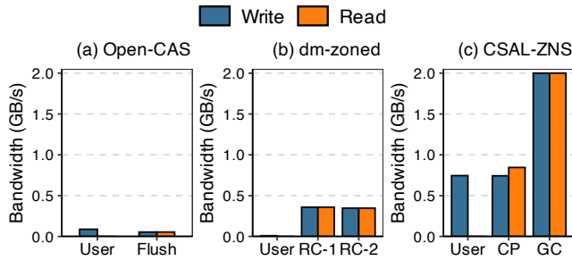
Figure 16. Backend Traffic under 4KB Random Writes. dm-zoned performs reclaiming from random to sequential zones (RC-1) and from sequential to random zones (RC-2). Open-CAS only performs flushing. CP and GC mean compaction and garbage collection.
